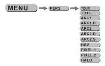
• Enter the [PERSONALITY] mode to select DMX mode: [TOUR], [TR16], [ARC1], [ARC1.D], [ARC2], [ARC2.D], [ARC2.S], [HSV], [PIXEL.1], [PIXEL.2], [HALO].
